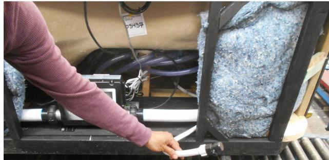
It is recommended to inspect the plumbing fittings plumbed through the control box to ensure all pieces are fully threaded in. unions can loosen up due to vibrations in transit.
