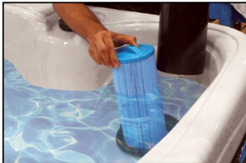
**NOTE: Make sure the filter has soaked at least 30 minutes before you install it. Insert the filter all the way and screw it in. Do not over-torque the cartridge during installation, just hand tighten gently.**
