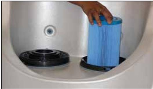
Unscrew the cartridge and remove it.
