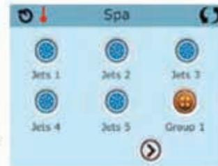
If the Spa has a Circ Pump, a Circ Pump Icon will appear to indicate its activity, but outside of Priming Mode, the Circ Pump cannot be controlled directly.
