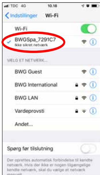
1. Before starting, ensure the wifi module is connected to the BP control pack. Also flip your spa breaker off then back on again to send the wifi module into discovery mode.
