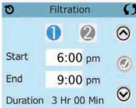
Press "1" to view Filter 1. Press "2" once to view Filter 2. Press "2" again to turn Filter 2 ON or OFF.
